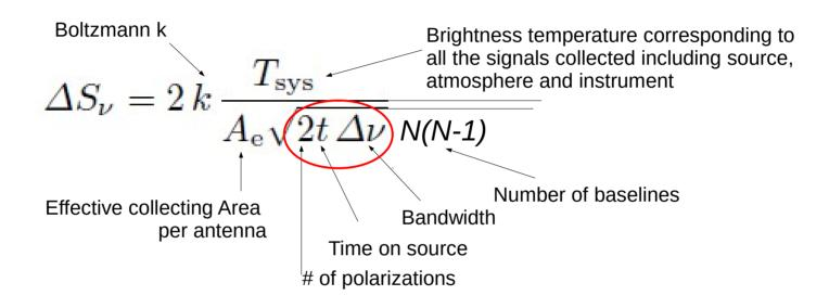
Sensitivity can be increased by increasing the bandwidth and/or the integration time
