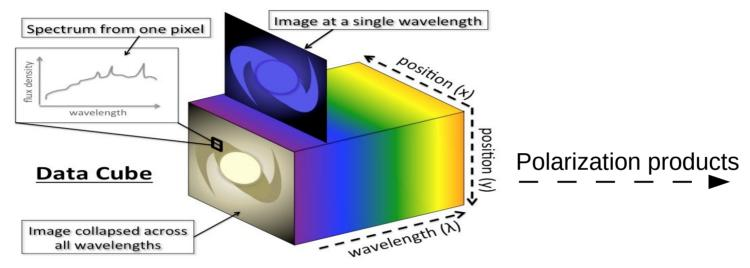
Continuum bandwidth is as large as 7.5GHz/pol The finest spectral detail you want to observe determines your resolution in the ranges from 0.1-111 km/s at 84 GHz to 0.01 - 10 km/s at 950 GHz.
