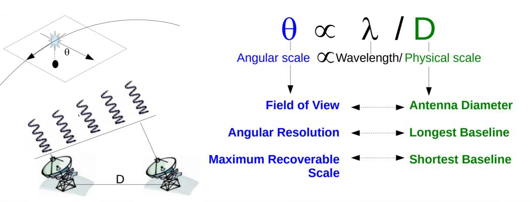
Angular scales not sampled by the available couples of antennas are filtered out
