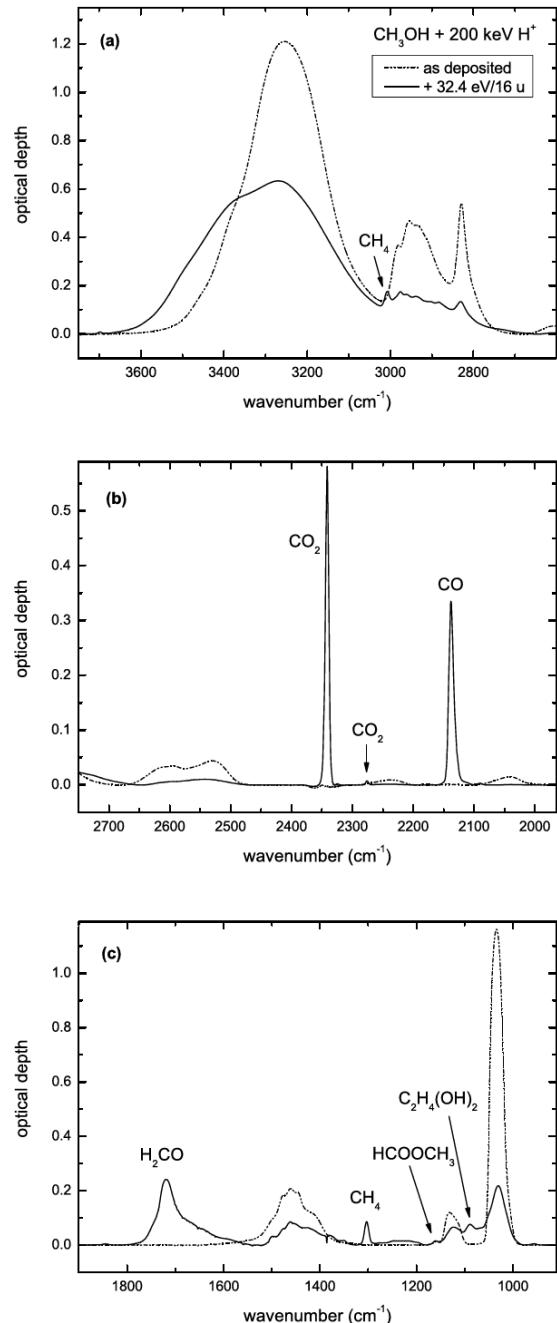
**Fig. 8.** Infrared spectra of a  $\text{CH}_3\text{OH}$  pure ice as deposited (dotted lines) and after irradiation with 200 keV protons (solid lines) in three different spectral regions from 3700 to 900  $\text{cm}^{-1}$  (2.70–11.11  $\mu\text{m}$ ).
