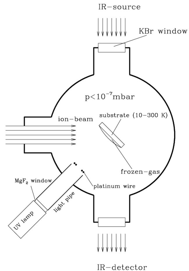
The sample is processed by energetic ions (200-400 keV) and by UV photons separately or simultaneously.
