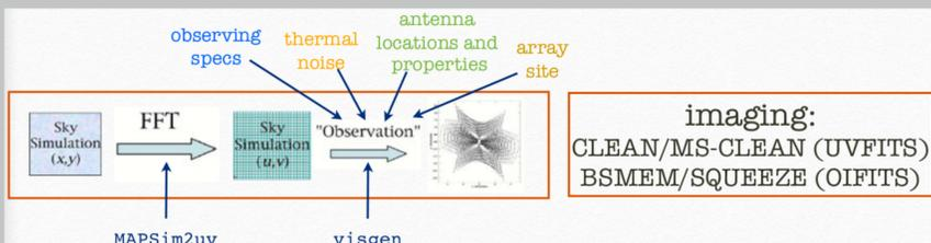
Figure 1 : Schematic overview of the steps executed in MAPS to reconstruct an input brightness distribution. The input is first Fourier transformed (MAPSim2uv) before visibilities are generated in the  $(u, v)$  plane (visgen), depending on the observational parameters. These can then be imaged with imaging softwares.
