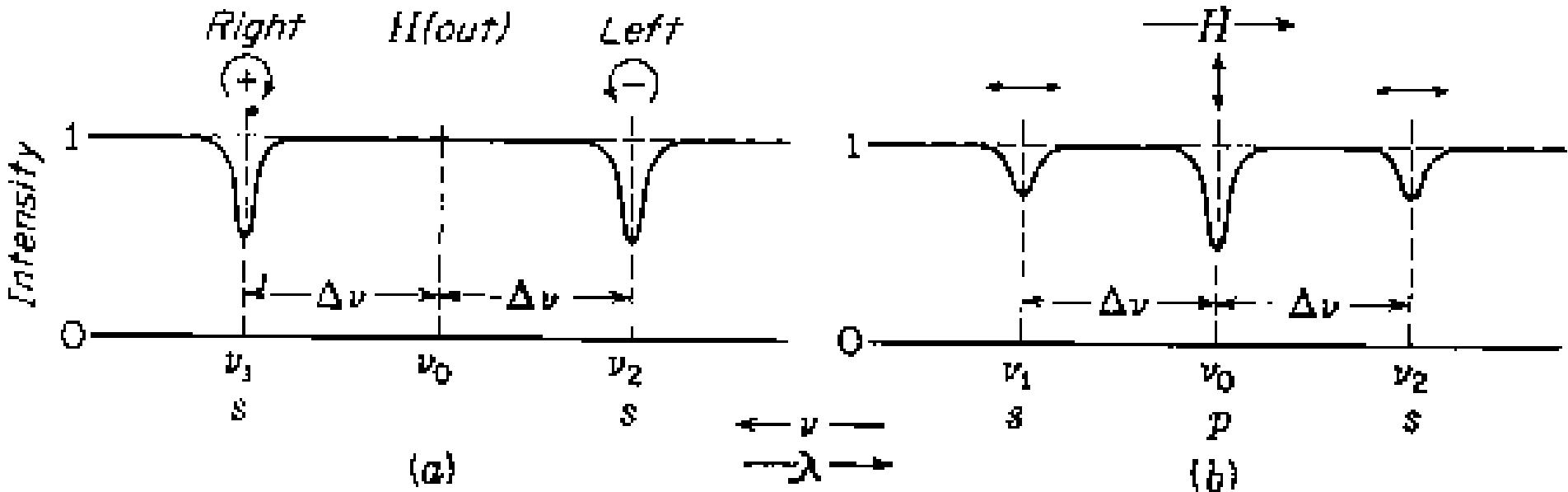
$$\Delta v_z = |\mathbf{B}| Z, Z \approx 1 - 2 \text{ Hz}/\mu\text{G}, (Z_{\text{HI}} = 1.4 \text{ Hz}/\mu\text{G})$$
