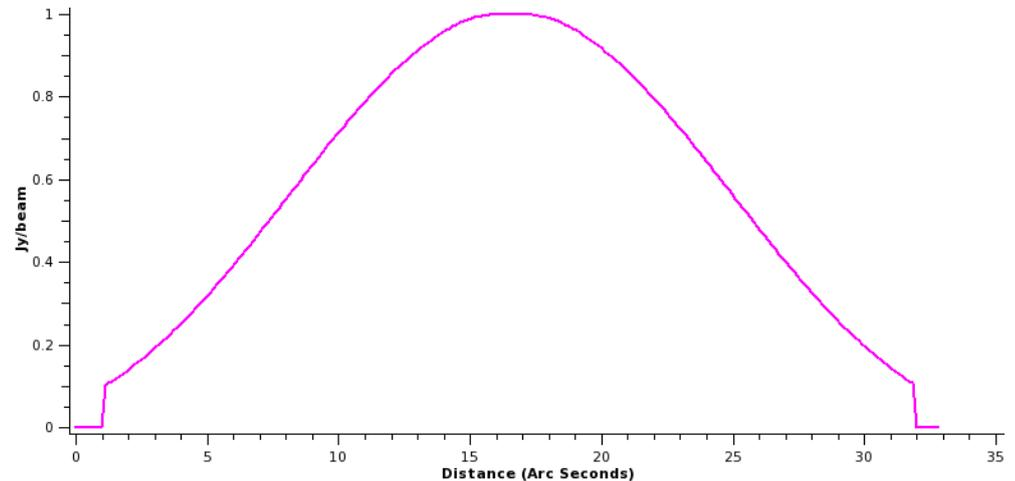
The response of the antennas in the array must be corrected for during imaging to get accurate intensities for source outside the core of the beam.
