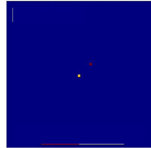
The Fourier transform FT of the sampled visibilities gives the true sky brightness convolved with the Fourier transform of the sampling function (called **dirty beam**).
