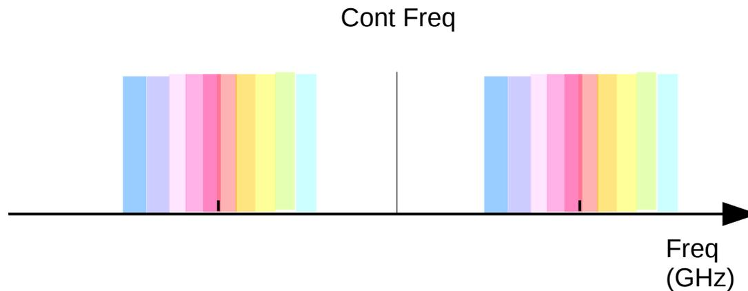
Modern interferometers use large band receivers. Data are taken in multichannel mode regardless if they are meant for continuum or line observations.
